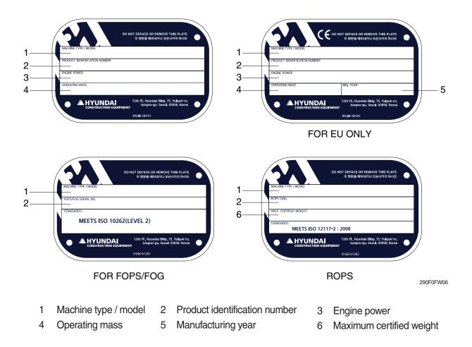
\* The machine serial number assigned to this particular machine and should be used when requesting information or ordering service parts for this machine from your authorized HD Hyundai Construction Equipment dealer. The machine serial number is also stamped on the frame.
